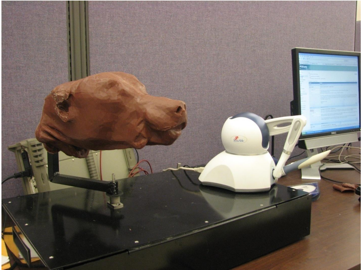
Figure 1: Physical System – Mannequin on top of the stand (black box). Inside the stand is a rotational sensor.
