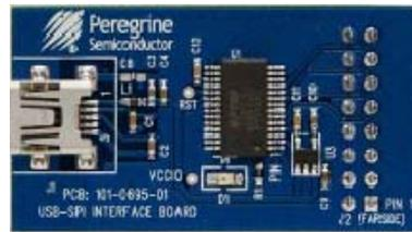
Figure 3. DSA USB Interface Board Connected to the PE4312 Evaluation Board for Latched Parallel and Serial Programming
