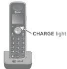
3. Charge the handset by placing it face up in the charger. The **CHARGE** light is on when charging.
