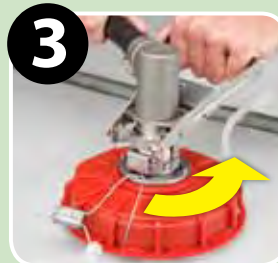
3 Turn Handle Counter-Clockwise
