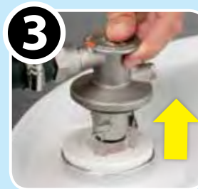
3 Pull Coupler up & Remove
