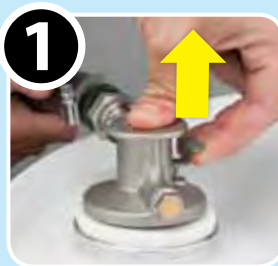
1 Pull up Lever on Side of Coupler
