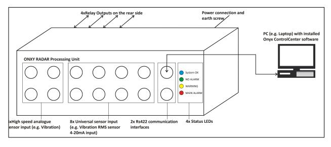
This system comprises 4 high-speed signal inputs, 8 universal signal inputs and 4 relay-outputs. For the power supply a voltage of 115...230V, 50/60Hz, 10W is needed and for configuration of system parameters a serial RS422 communication to a PC which is running the ONYX CONTROL CENTER software is needed.
