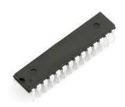
The Micromite is a low cost Microchip PIC32 microcontroller programmed with the MMBasic firmware.
