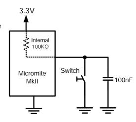
mechanical assembly. Because the Micromite runs very fast a BASIC program could see this as a secession of quick button presses rather than a single press.
