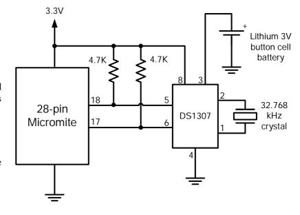
RTC SETTIME command which uses the format RTC SETTIME year, month, day, hour, minute, second. Note that the year is just the last two digits (ie, 15 for 2015) and hour is in 24 hour format.
