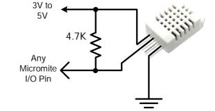
To get the temperature or humidity you use the HUMID command with three arguments as follows:
