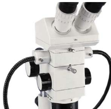
Picture 13: Bright-field incident light illumination, cold light device
