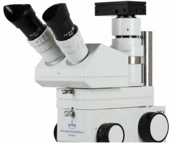
Picture 29: SMT 4 with TV-adapter 0,63x and USB camera
