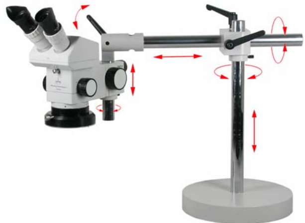
Picture 34: Assembled SMT 4 at column stand
