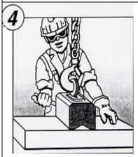
Position of wasting device at the center of gravity of the park to be lifted
