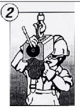
Check the condition of the hoisting device
