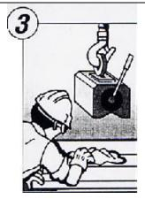
Clean the poles and the surface of the parts in contact with the hoisting device. File any burrs.
