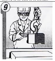
Carefully set the part down. Bring the lever to the OFF position to demagnetize the part. Slowly raise the hoisting device ensuring that the part is detached.
