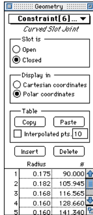
Figure 4-9 Geometry window for a curved slot
