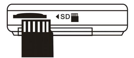
3) System memorizer will automatically be set up as Mini SD card after insert it.
