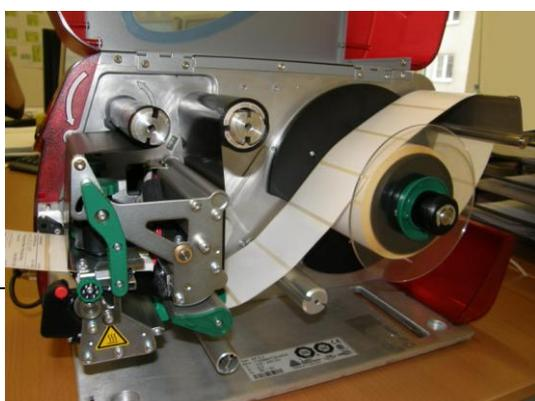
Now release the green handle (counter-clockwise) and insert the label roll as shown. Make sure the carrier foil is adjusted to the left.
