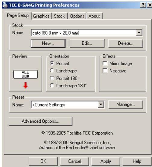
In the "General" section, click "Printing Preferences" and create a new label template by clicking "New" and then enter "80.0" for width and "50.0" for height. Set margins to "0". For the name, enter "cato".
