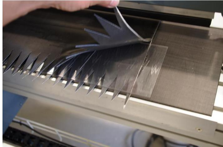
Once the anti-cut plate has been placed inside, we insert the material up to the second mark
