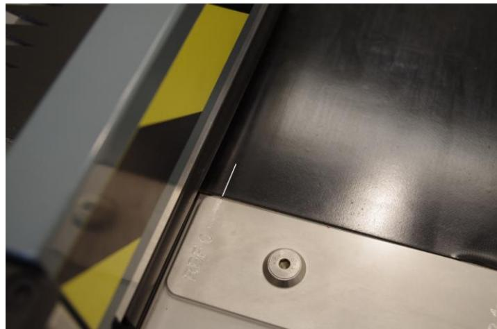
We reduce the cutting pressure to 2 bar, as the second cut shall only cut the top fabric.
