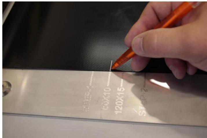
We then place the belt under the tread bar until the mark made matches up with 0 Ref. and we make sure it is fully in contact with the guide rail.
