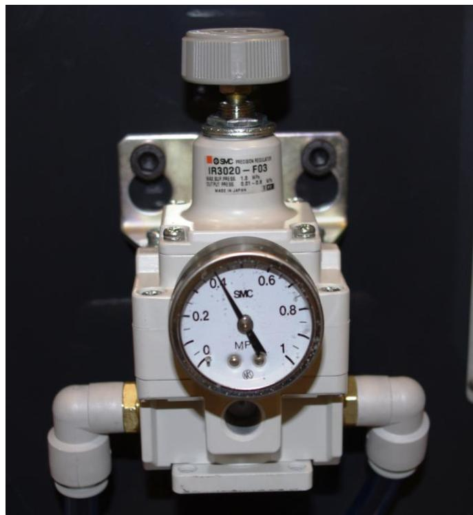
This adjustment device suffers a loss of air to maintain constant the exact pressure
