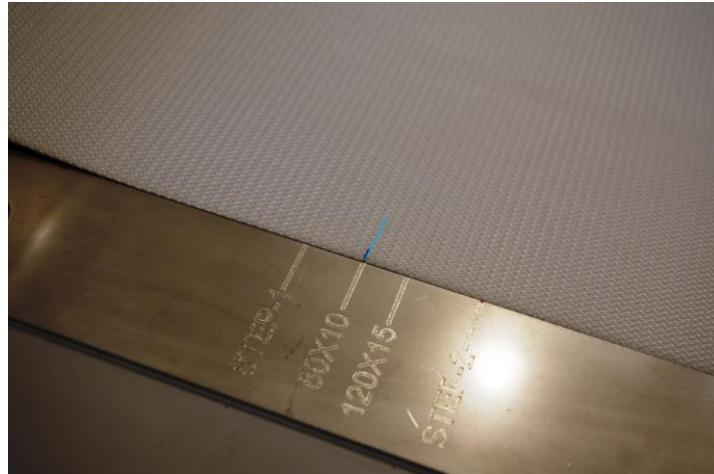
We then feed in the belt under the holding bar until the mark made aligns with 0 Ref. and we make sure it is fully in contact with the guide rail.
