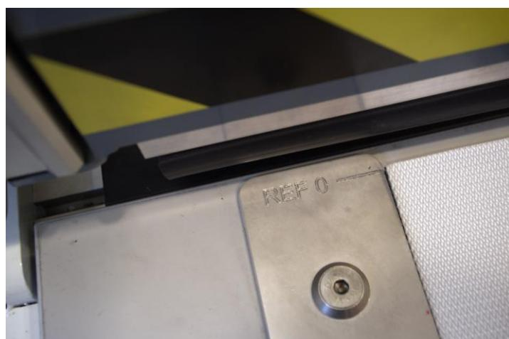
Then mark the measurement to feed in the material with a pencil, according to the die one wishes to use.
