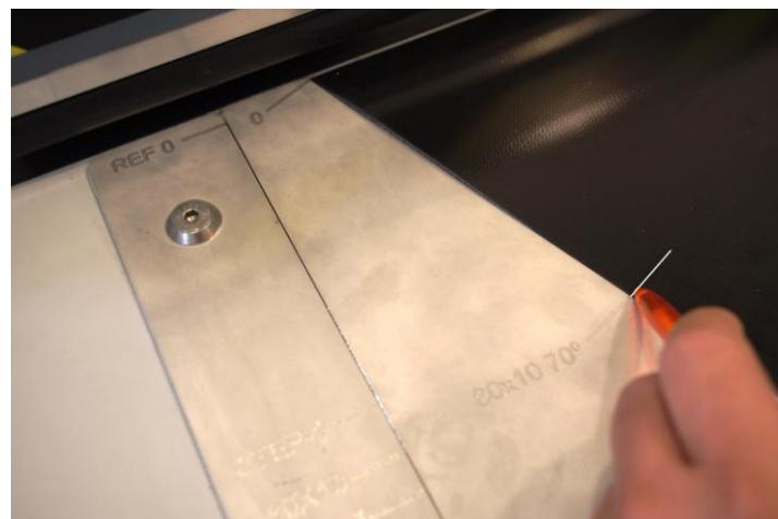
We then insert the belt until it aligns with the mark made at point 0 Ref.
