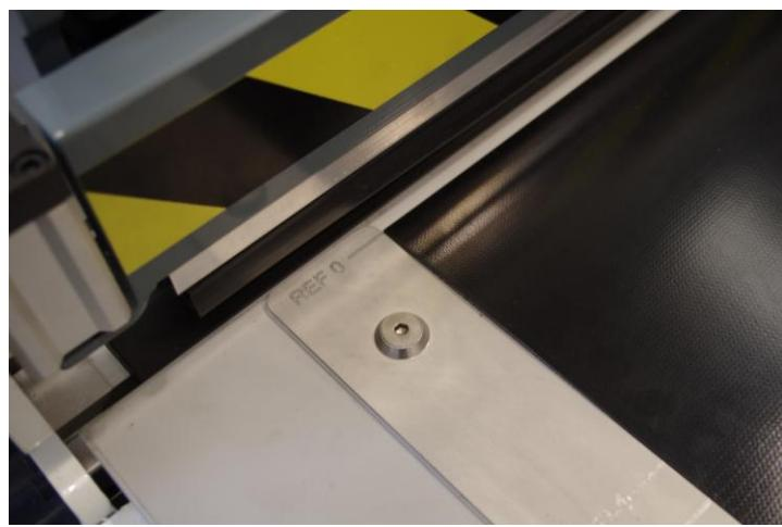
We then place the belt under the holding bar until the mark made aligns with 0 Ref. and make sure that it is fully in contact with the guide rail.
