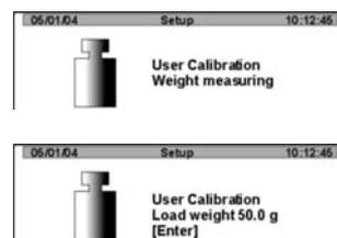
⇒ Now place the adjusting weight in the center of the weighing plate, press the
