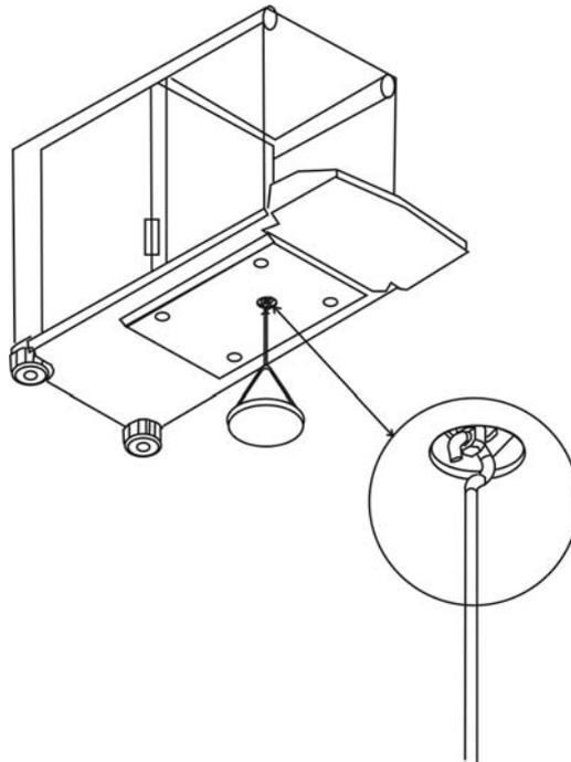
Fig. 1: Setting up balance for under floor weighing
