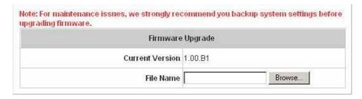
Warning: 1. Firmware upgrade may cause the loss of some of the data. Please refer to the release notes for the limitation before upgrading the firmware. 2. Please restart the system after upgrading the firmware. Do not power on/off the system during the upgrade or the restart process. It may damage the system and cause it to malfunction.
