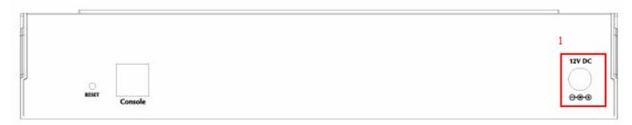
Connect the 12V DC power adapter to the power connector socket on the rear panel. The Power LED should be on to indicate a proper connection.
