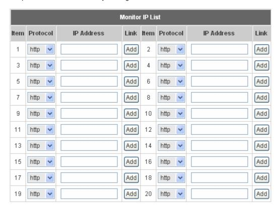
When "Monitor" button is clicked, Monitor IP Result page will show up. If the entered IP address is unreachable, a red dot under Result field will appear. A green dot indicates that the IP address is reachable and alive..
