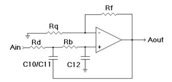
For the MOTM-485 circuit, think of Rd as the diode bridge Q10, Rb as R48, Rf as R47 and Rq as the R23+R37+TP1+C9+Q7 chain. Yes, there is a capacitor in there (never mind a transimpedance diode cell made from Q7) but we're dealing with AC impedance so think of it as a resistor. It is much easier that way. The op-amp? We'll get to that.
