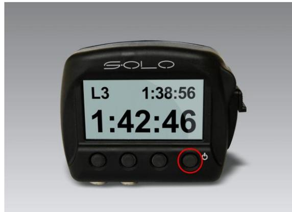
In case of **Solo externally powered**, AIM recommends to connect it to the vehicle master switch so that the logger switches automatically on when the vehicle is powered and off when the vehicle switches off.
