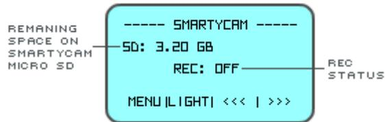
To enable this page follow this path: MENU>>Display Setup>>Enable/Disable Pages, scroll until finding SmartyCam page: after having enabled it, you can look at it and scroll the pages using VIEW button.
