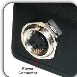
**SoloDL** features two connectors on the bottom of the system: one to connect to an external CAN expansion (for example SmartyCam – see Chapter 11) and the second is used for ECU connection and power (bottom right image). Please, take note that the external power can be received from the first or the second connector.
