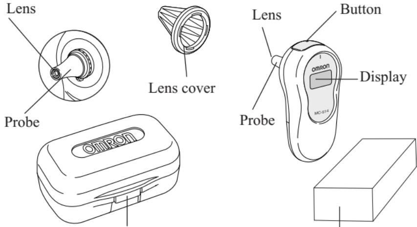
Storage case (with 10 lens covers inside, plus 1 on the thermometer)      Box for lens covers (with 10 lens covers inside)
