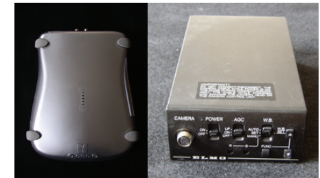
Fig. 2: Video digitizer (VD) and Video Control Box (VC)
