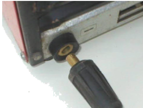
Figure 13: Negative Cable Connection
