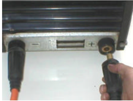
Figure 14: Positive Cable Connection
