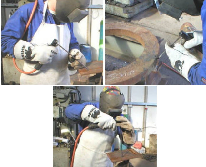
Figure 20: Preparing to Cut
