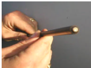
Figure 19: Connect Electrode to Stinger
