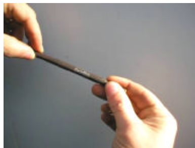
Figure 18: Check Cutting Electrodes for Damage
