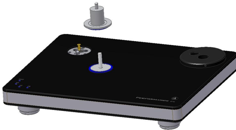
Pic. 4: Fitting the bearing upper part
