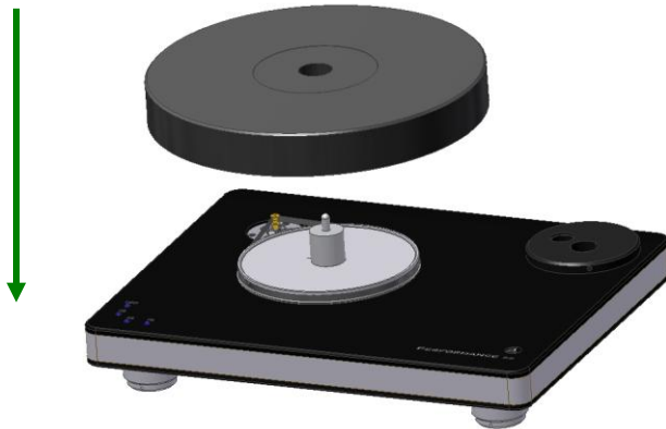
Pic. 6: Setting the platter onto the bearing
