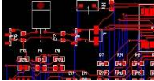
Figure 9.3 Power supply distant from rest of circuit
