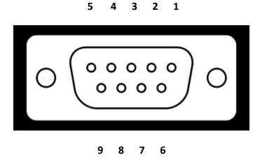
The function of each pin is described below. The pin-out follows the MODBUS specification for RS485 connections using this style of connector.
