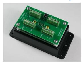
The optional PWS-400T Terminal Block accessory board attaches to the 9-pin connector of the PWS-420 and provides terminal block connections for wiring all signals. A switch is provided on the board to implement the Bluetooth radio wake-up function, simplifying wiring when a remote switch is not needed. A remote switch may be wired in parallel using the MODE and GND terminals of TB2. Optionally, a jumper can be wired between MODE and GND for continuous Bluetooth radio operation.
