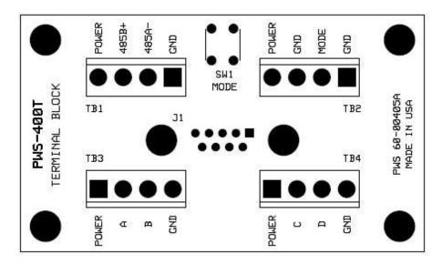
Note: Signals A, B, C, and D are not used on the PWS-420 and must be left unconnected.
