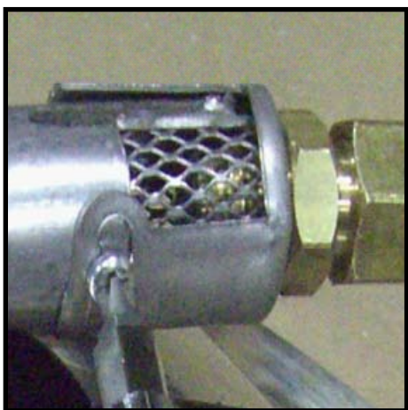
Step 3. Remove shutter screw and slide off.
