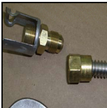
Step 4. Remove brass orifice from flex line.
