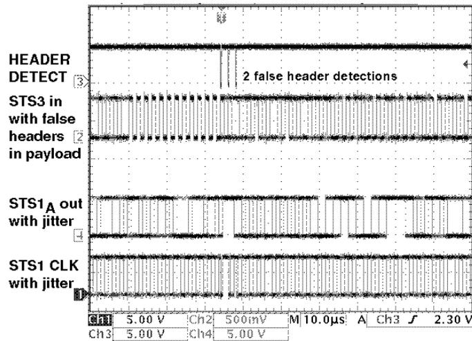
Fig.2b STS-3 DEMUX with FALSE HEADER DETECT set OFF
