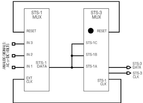
Fig. 2A STS-3 MUX with only one STS-1 MUX
