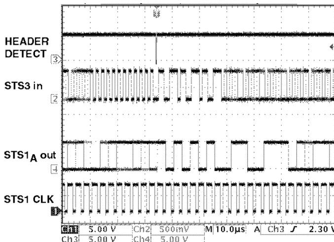
Fig.2a STS-3 DEMUX with FALSE HEADER DETECT set ON
