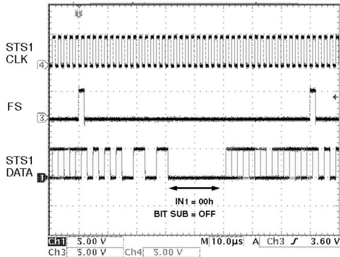
Figure 2a: TIMS STS-1 signals with BIT SUB off
