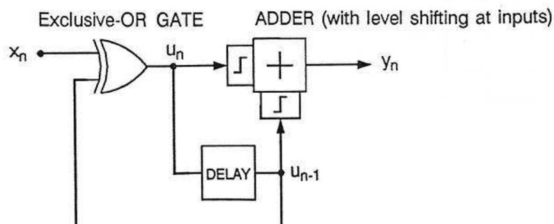
Figure LCE-1 Precoded Duobinary Model
