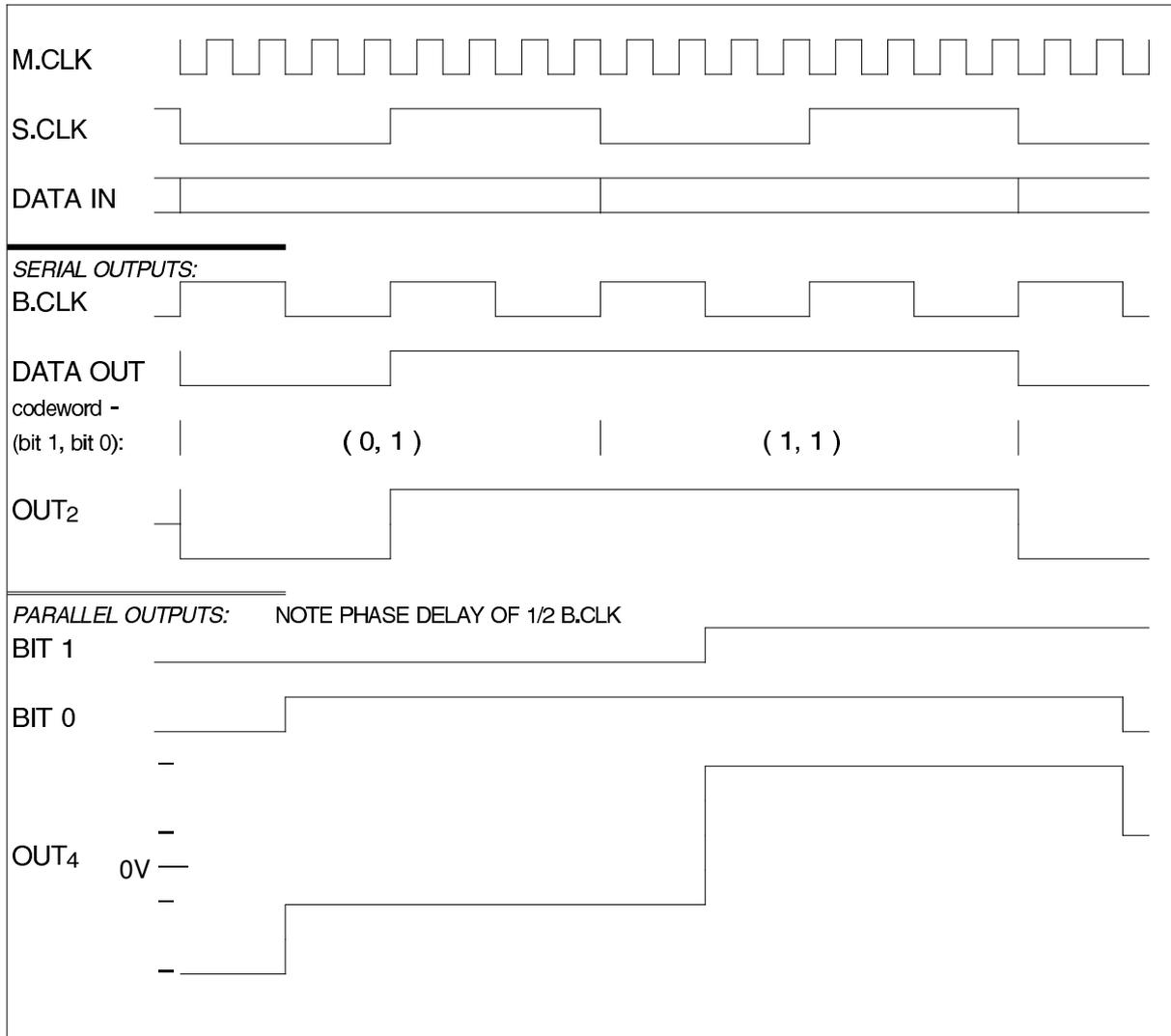
NOTE: The parallel output bits are delayed in phase with respect to the serial output bits by half a cycle of the bit clock, **B.CLK**.
