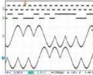
Fig.3b - CLK, DATA, i and q waveforms
