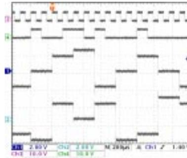
Fig.1b - CLK, DATA, i and q waveforms
