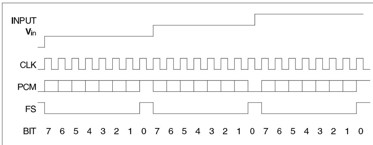
PCM ENCODER timing diagram
