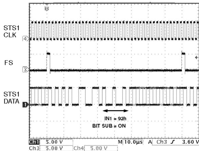
Figure 2b: TIMS STS-1 signals with BIT SUB on
