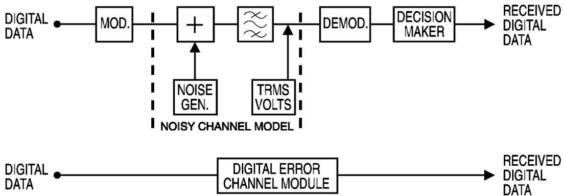
**Fig 1: DIGITAL ERROR CHANNEL module compared to the functional blocks which it can replace to simplify BER experiments.**
