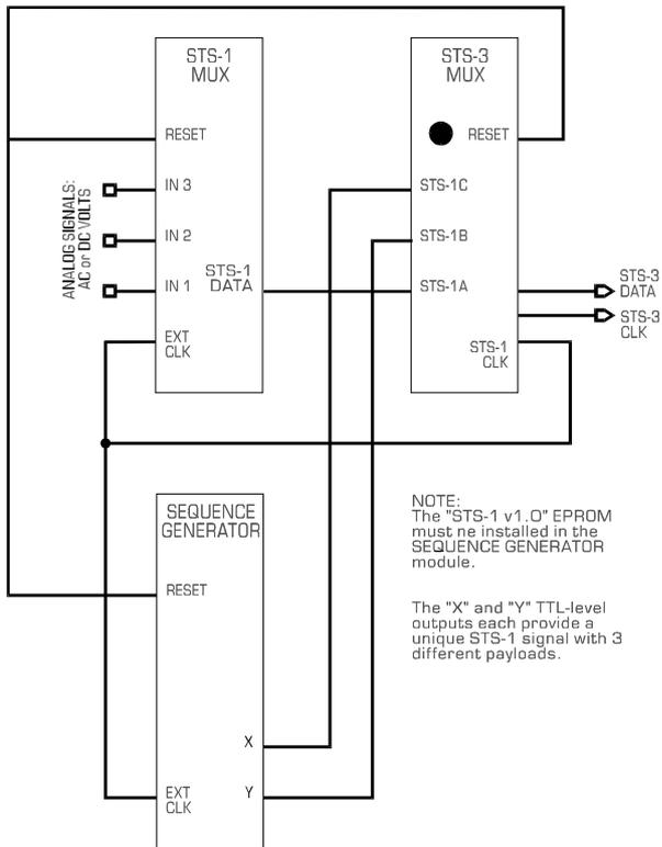
Fig. 2B STS-3 MUX with an STS-1 MUX & a SEQUENCE GENERATOR
