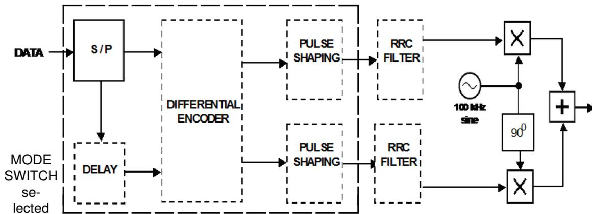
Fig.5 - Modulator Block Diagram.
