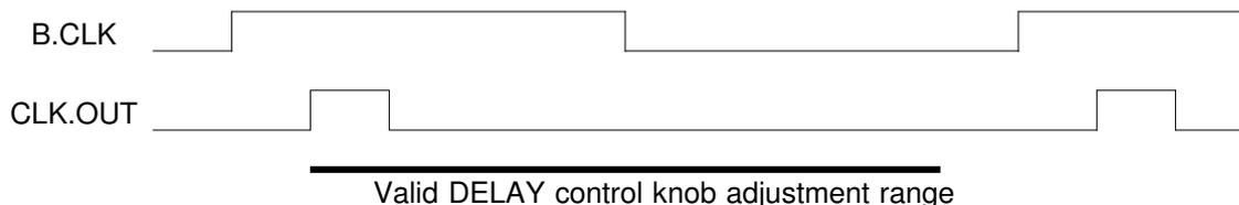
Caution: always ensure that the **CLK.OUT** pulse remains within the **B.CLK** cycle, as illustrated above. Extending the **CLK.OUT** pulse into the following cycle will cause invalid operation.
