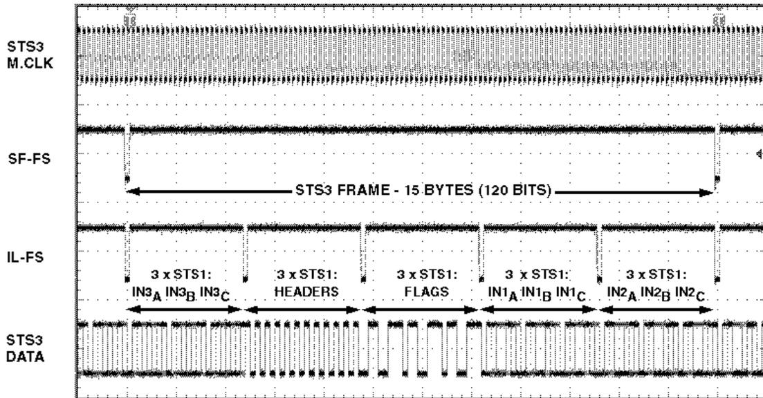
Fig.1 TMS STS-3 frame structure
