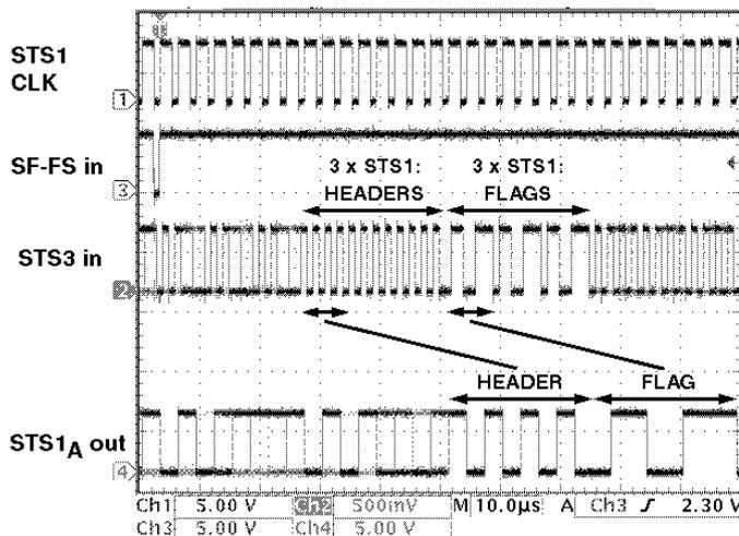
Fig.1 TIMS STS-3 DEMUX de-interleaving an STS-1 signal
