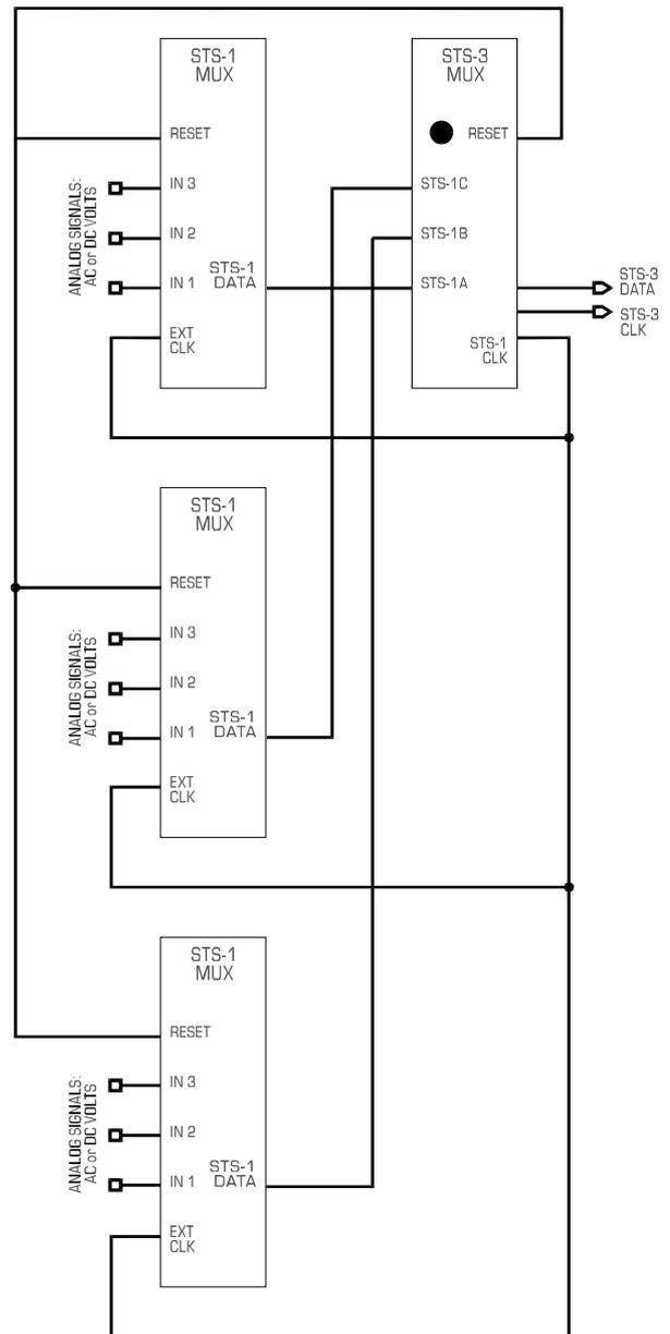
Fig. 2C STS-3 MUX with three STS-1 MUX modules
