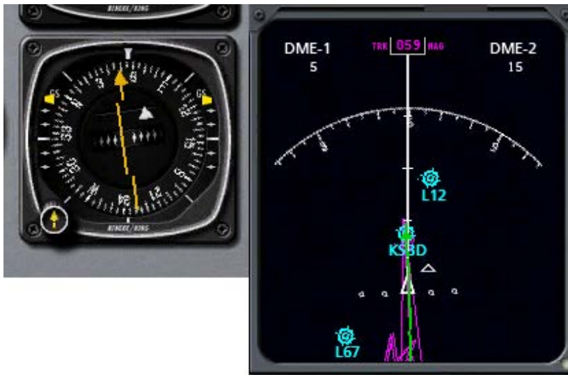
Figure 12.16: Tuning the CDI for the approach
