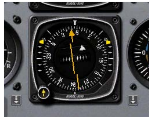
Figure 12.17: Reading the glideslope and CDI
