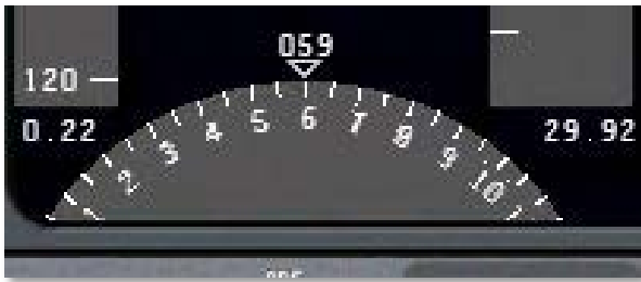
Figure 12.13: The directional gyro in the EFIS display
