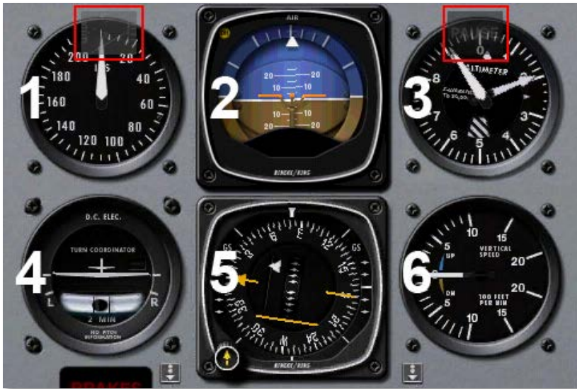
Figure 2.5: The steam gauge panel
