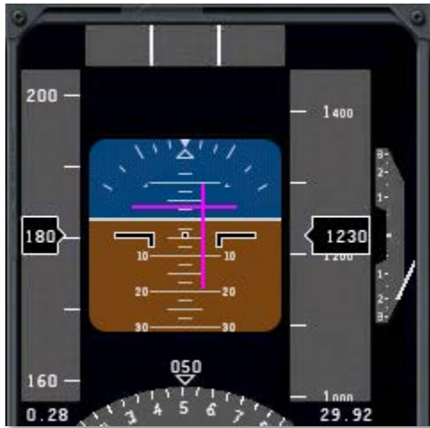
Figure 12.18: Reading the glideslope and CDI in the EFIS display
