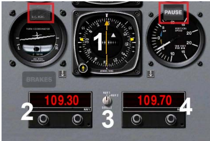
Figure 12.8: Navigation instruments in the steam gauge panel
