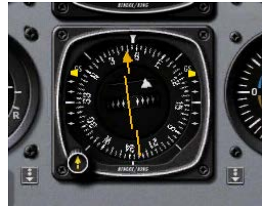
Figure 12.10: The CDI in the piston-engined aircraft
