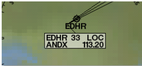
Figure 12.5: A LOC beacon
