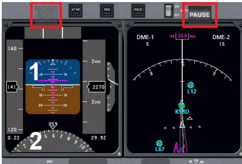
Figure 12.12: Navigation instruments in the EFIS panel
