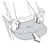
Slide the sides of the cover off the sides of the frame. Slide the harness through the slots in the sides of the cover.
