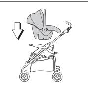
Slide the locking catches on sides of the chassis outwards and push the attachment brackets down. **Never place a child in the pushchair with the brackets up.**
