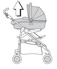
Slide the locking catches on sides of the chassis outwards and push the attachment brackets down. Never place a child in the pushchair with the brackets up.
