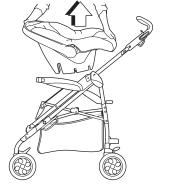
Align the locking clip of the car seat with the attachment brackets of the pushchair.
