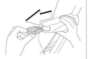
Insert the two ends of the bumper bar into the holes in the ends of the armrests. Push the bumper bar in until they click into position.
