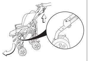
Ensure the handle in the centre of the pushchair's back is pushed down as far as possible by gently pushing the lever plates at the back fully down.
