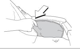
Unfasten the press studs at the bottom of the wings of the backrest.
