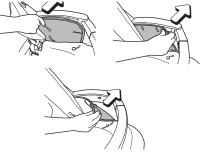
Fasten the sides of the cover to the chassis armrests as shown in the diagrams.
