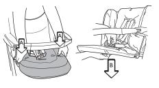
Place the cover and backrest onto the seat of the chassis as shown in the diagram.
