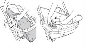
Finally, pull the cover off the back of the pushchair.
