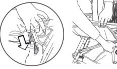
Fasten the front of the cover to the chassis using the press studs.
