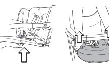
Push the two attachment brackets down until they click into place on the braces. Check they are fully attached by attempting to pull them out again
