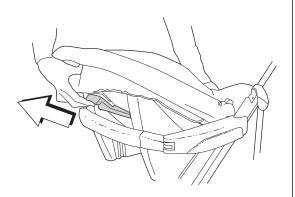
In the corners of the seat of the chassis are there are two attachment brackets. Rotate the attachment brackets upwards as far as they will go. The brackets will lock in a vertical position.
