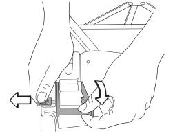
In the corners of the seat unit where the backrest joins the seat base there are two flaps. Under the flap are the attachment brackets. Rotate the attachment bracket upwards as far as it will go. The bracket will lock in a vertical position.
