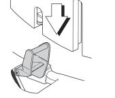
Push the car seat down onto the attachment brackets until it clicks into place. Check the car seat is firmly in place by attempting to lift it upwards.
