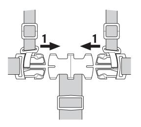
Unlocking the harness: Squeeze the ends of the tongues together (2) and then slide them out of the buckle (3). Your child can now be removed from the pushchair.
