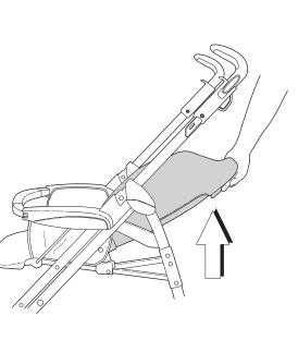
To adjust the leg rest, pull the locks on both sides of the leg rest in the direction of the arrows in the diagram. Now either lift or lower the leg rest, the leg rest will lock automatically into position.
