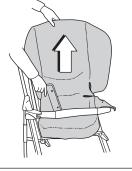
Repeat the same process to remove the rear attachment studs from the armrests.
