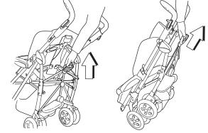
Ensure that the two locking catches below the finger catches lock over the clips on the rear leg attachment moulding, as shown in the diagram.
