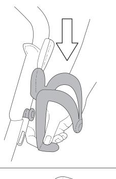
Continue to push the cup holder down onto the attachment point until it 'clicks' into position. Never place items weighing more than 0.5 Kg (1lbs) in the cup holder.
