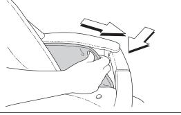
Unfasten one side of the harness by removing the screw as shown in the diagram, you will need to hold on the other side of the frame with your fingers.
