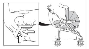
Still holding the lock up, lift the carrycot clear of the pushchair. Once the carrycot has been removed always refit the bumper bar, *see page 9*.
