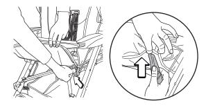
Push the buttons on the two backrest attachment brackets inwards and hold.
