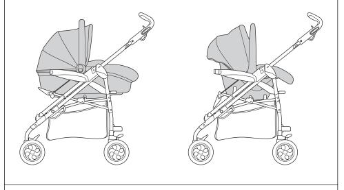
The chassis can also be converted into a pushchair by attaching the backrest and fabric cover (see pages 14 to 15 for fitting instructions).
