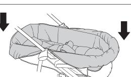
Fasten the press studs on the backrest end of the liner to the two press studs on the on the back of the backrest.
