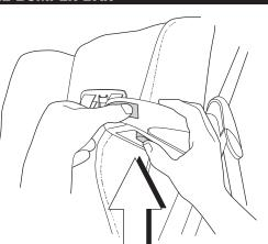
With the button still pushed in, slide the cap out of the armrest. Repeat the process for the other armrest.
