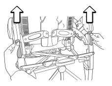
Press the buttons on the ends of the backrest inwards (1). Lift the two ends of the backrest out of the attachment brackets at the back of the chassis (2).
