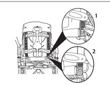
Attach the backrest adjusters to the rear legs of the chassis. Turn the attachment brackets on the backrest adjusters upwards (A). Align the attachment brackets with the braces on the pushchairs rear legs (B).
