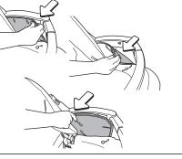
Slot the end of the crotch strap through the seat of the chassis and the slot in the seat cover.
