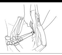
Unfasten the two press studs holding the seat fabric to the frame. Gently slide the cover off the front of the footrest.
