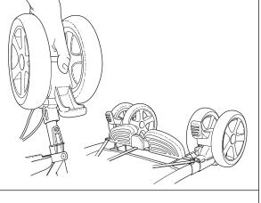
Check that the pins in the pushchairs legs are protruding through the wheel housings. Check the wheels are correctly fitted by trying to pull them off again.
