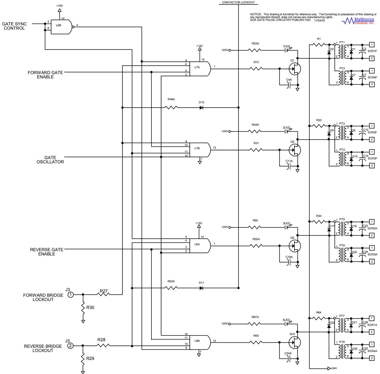
Figure 12: SCR Gate Pulse Circuitry
