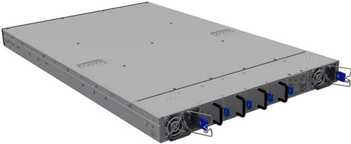
Figure 5: Unlocking the Latches and Extracting the PSU
