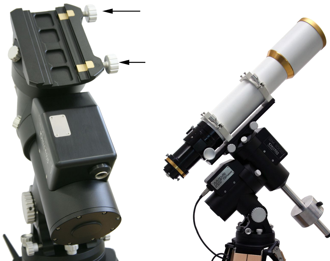
Fig. 4.14: Safety position. Note the position of the dovetail locking knobs on the right of the mount (marked by arrows).
