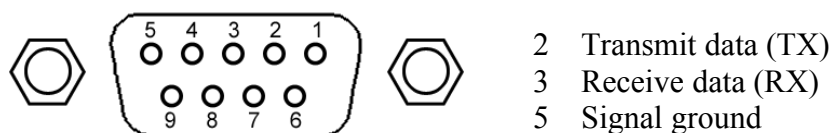
Fig. 5.2: RS-232 port pinout.
