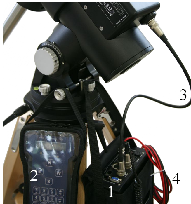
Fig. 5.8: Electrical setup. 1 – control box; 2 – hand pad; 3 – mount cable; 4 – power supply cable.
