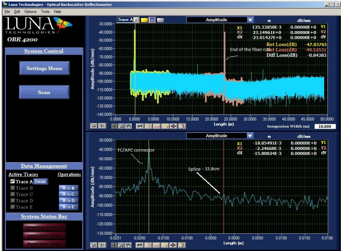
Figure 5.12 OBR display for a splice [12]
