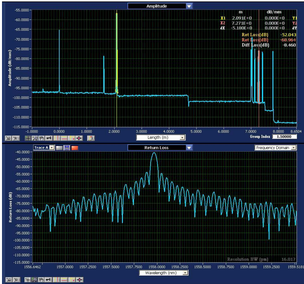
Figure 4.6. Return loss in the frequency domain (bottom plot) based on highlighted section of data in the time domain (top plot). [11]
