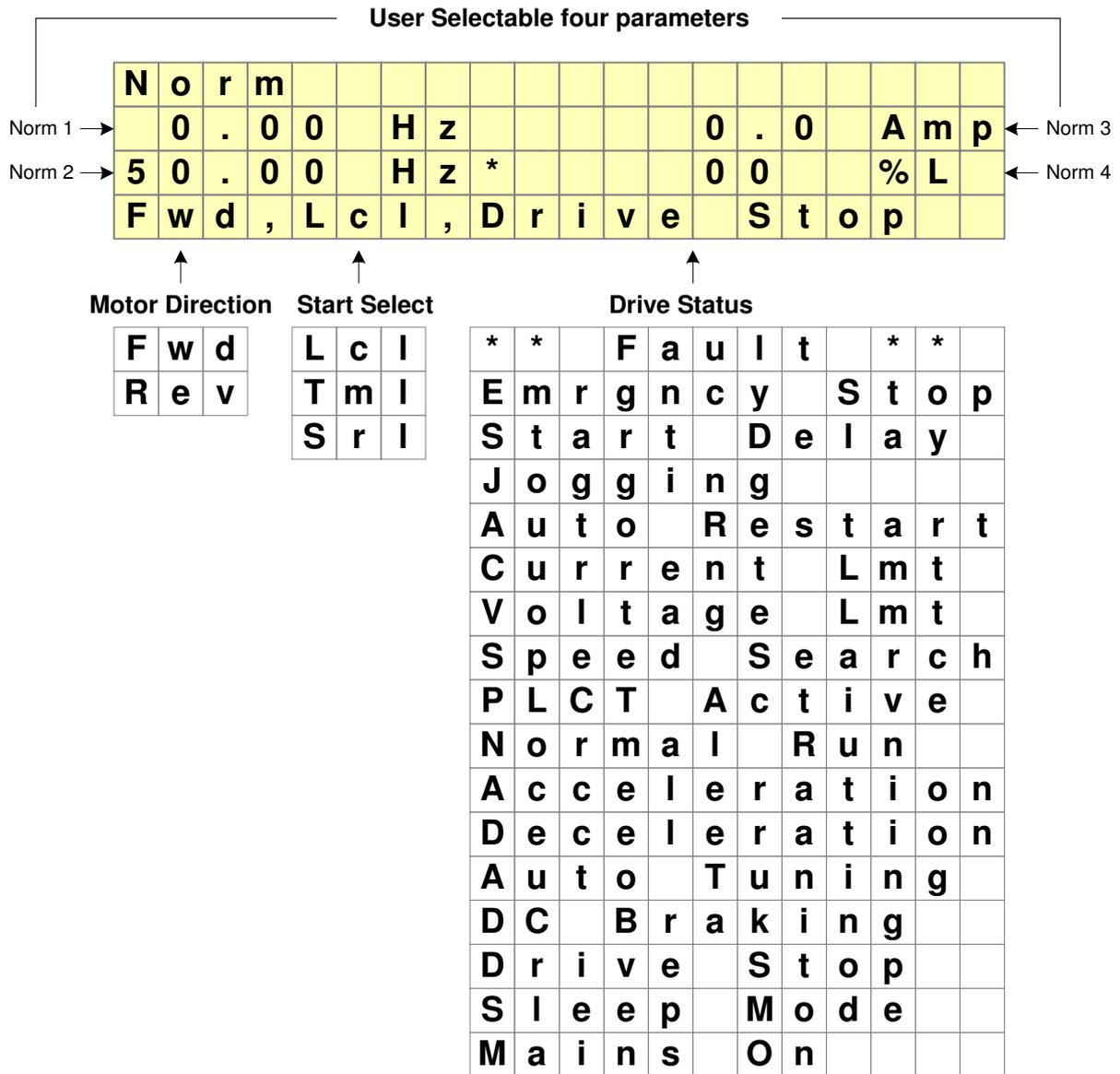
The above figure also indicates the selected direction of rotation, start selection and drive status. The four user selectable parameters can be configured using A601 ~ A604.
