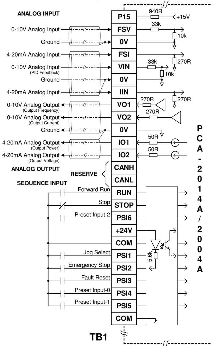
(Sink logic operation is considered for programmable sequence inputs in this diagram)
