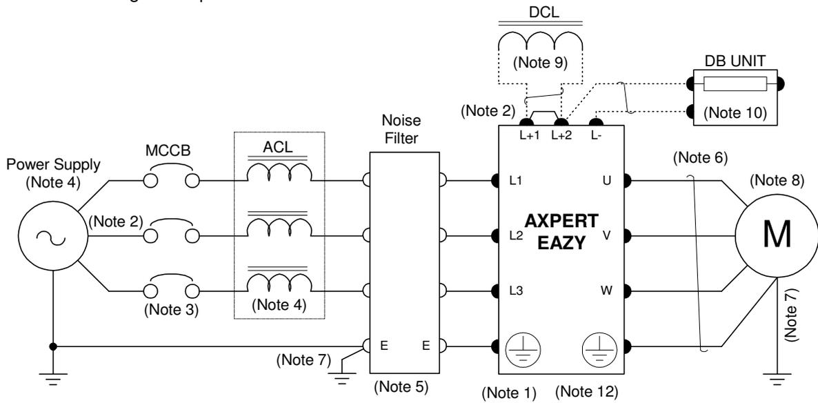
**EXAMPLE OF MAIN CIRCUIT WIRING**
