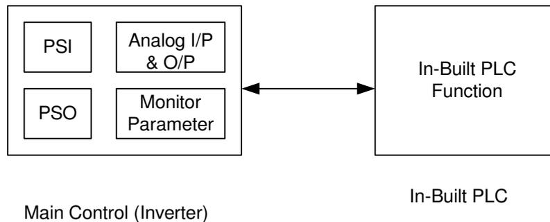
**Fig. 6-2 Block Diagram Of In-built PLC function with Main Control**
