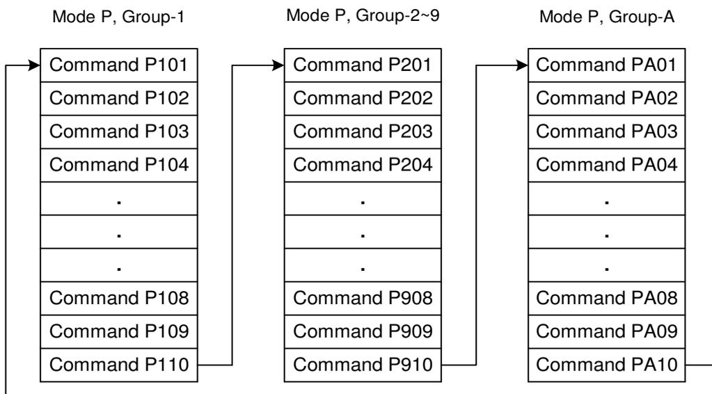
**Fig. 6-1 In-built PLC processing Chart**
