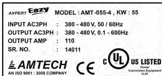
Observe the following matters when using the inverter as an UL/cUL Standard compatible product.
