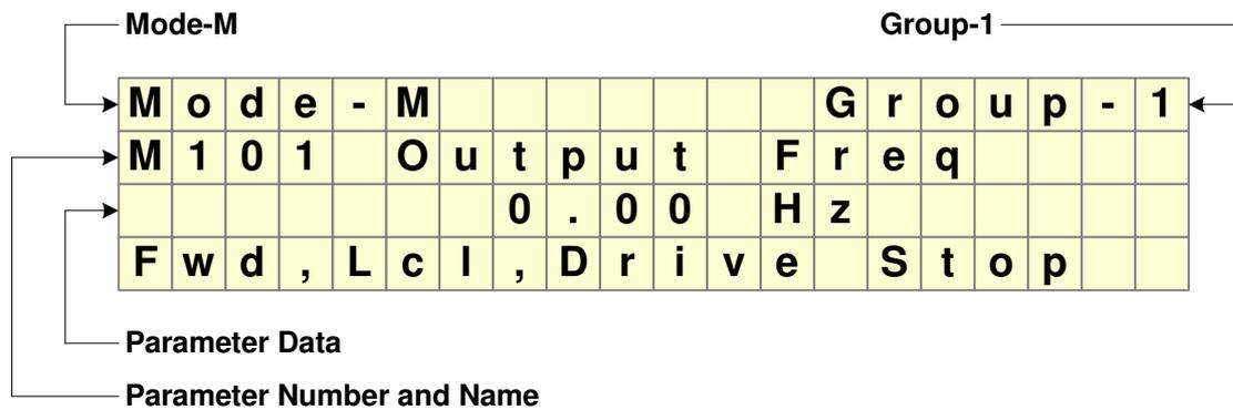
The first line indicates the present mode and group. The second line indicates the parameter number with its name and the third line shows its value. The fourth line shows the present status and remains all the time except fault condition, contact information and fault history.
