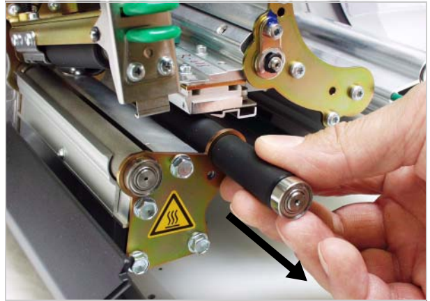
[3] Replacing the print roller
