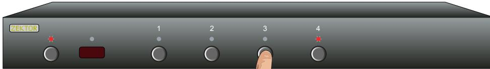
After '3' is pressed, the standby LED continues to flash, and the front panel will display the current Light Mode setting.
