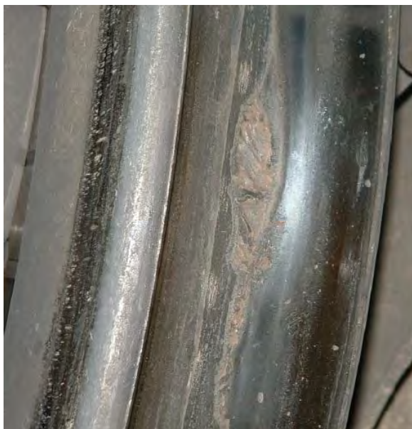
Photograph 29 badly turned wheel resulting from impact from foreign object
