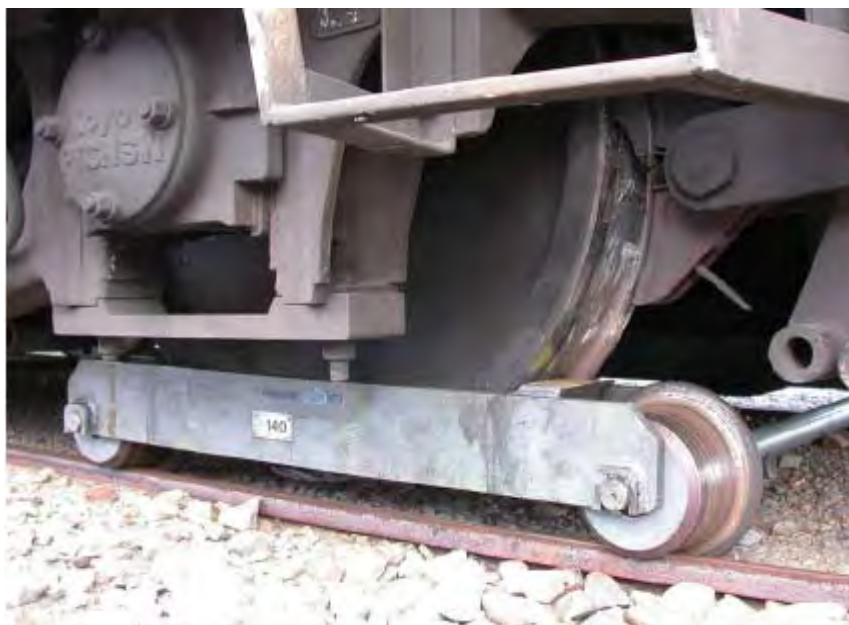
Photograph 30 Pony bogie assembled and in position
