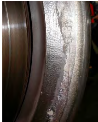
Photograph 8 Sub surface fatigue crack (extending to back of wheel)
