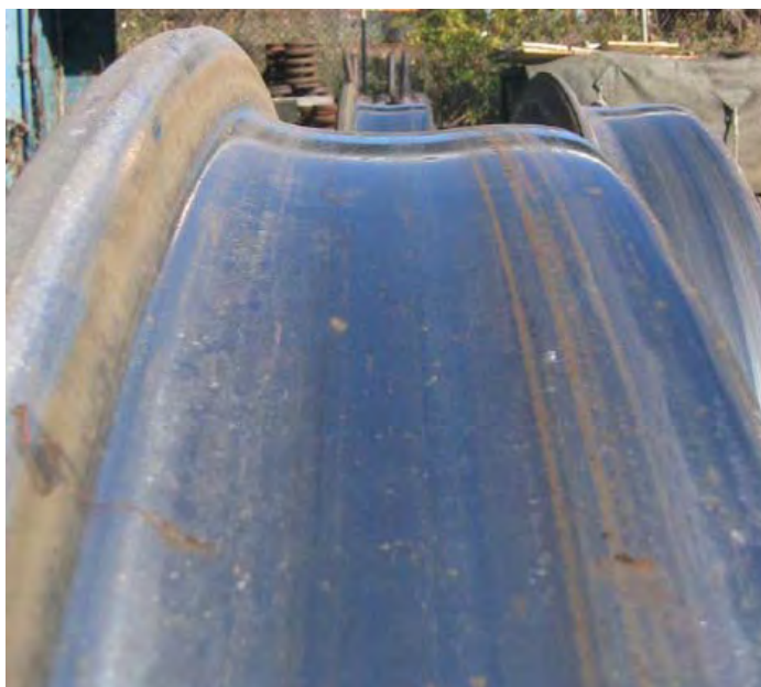
Photograph 25 Tread wear showing hollow tread
