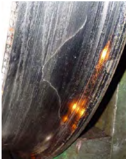
Photograph 7 Sub surface fatigue crack (identified during wheel turning)
