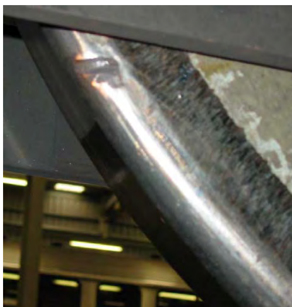
Photograph 28 badly turned wheel resulting from impact from foreign object
