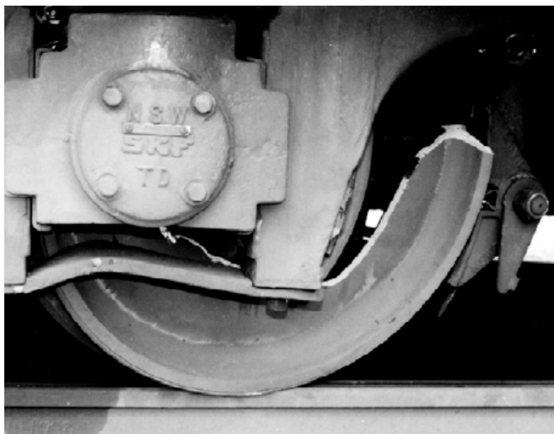
Photograph 5 Fractured wheel caused by thermal crack
