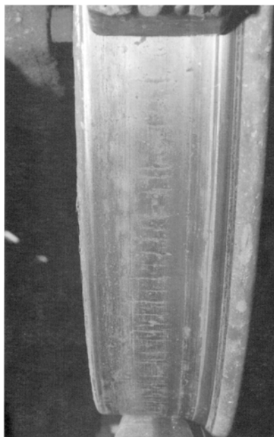
Photograph 1 - Class 2 thermal crack
