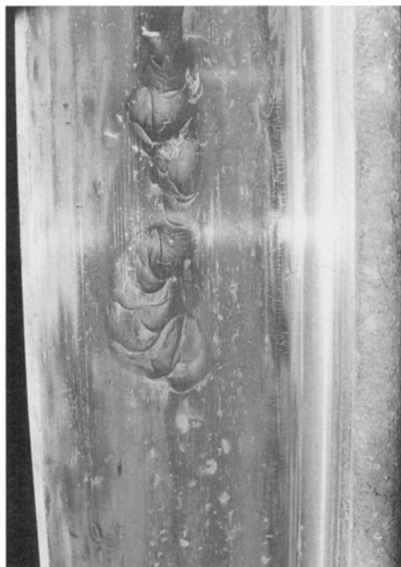
CLASS 3 SKIDDED WHEEL (MULTIPLE CLASS 2 SINGLE SKIDS)
