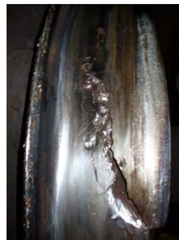
Photograph 10 Sub surface fatigue crack propagated to surface
