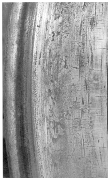
Photograph 3 - class 4 thermal crack
