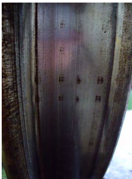
Photograph 26 badly turned wheel resulting incorrect turning process
