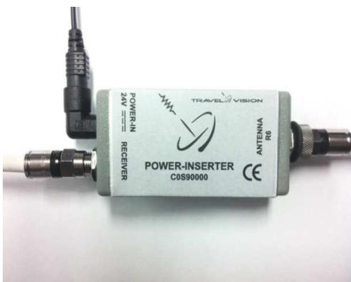
Press the F-connector on the other end of the coaxial cable over the connector of the power inserter (indicated with "Antenna R6"), so that the rubber is indented, and hand-tighten it.
