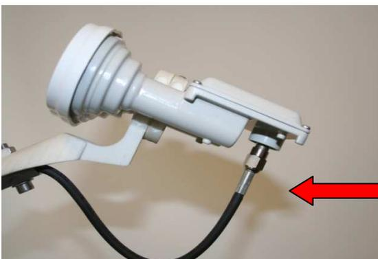
Before using the system, connect the cable with the F-connector to the LNB and hand-tighten it. No tools are required.
