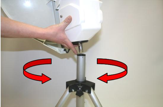
Guide the rotation axle of the antenna dish into the plastic socket of the tripod
