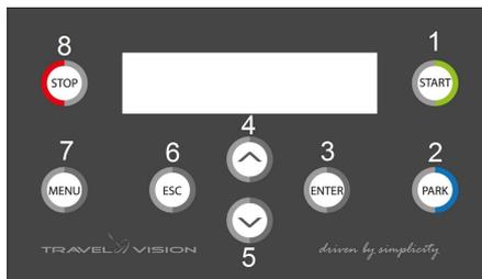
You can browse through the preprogrammed satellites step by step. By means of the arrow buttons located on the control module (buttons 4 and 5), For each satellite, the correct LNB position is shown on the display.
