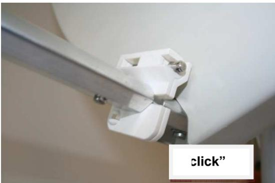
Ensure that the arm locates into its hinge ensuring that the LNB is properly aligned with the antenna dish.
