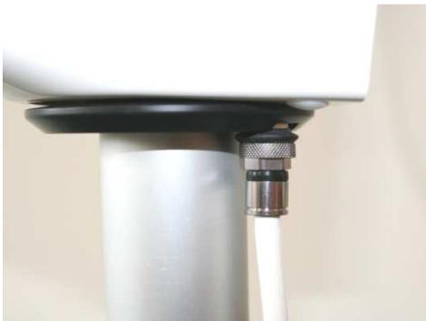
Firmly press the F-connector of the coaxial cable over the connector located on the bottom of the dish unit, so that the rubber is indented, and hand-tighten it.
