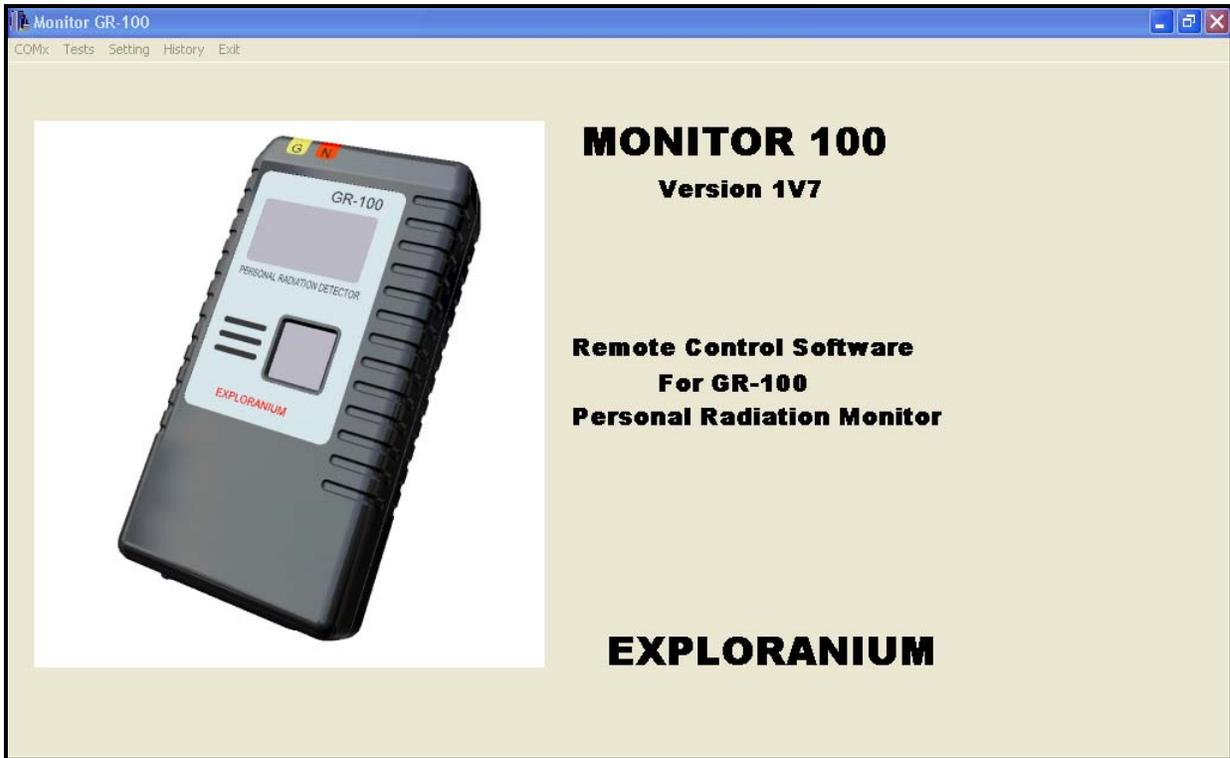
Four menu items are available in the menu bar, three of which are for controlling the unit: Tests, Setting and History. The Exit button stops the program. To switch among the Tests, Setting and History screens, you have to return to the main menu first by clicking on the Main Menu Button.
