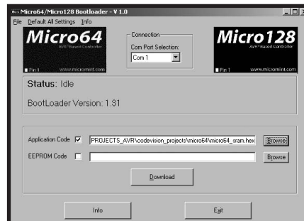
Photo 5 —It doesn't get much easier than this. Just compile your code into a hex file, point to it, click the Download button, and reset the Micro64.
