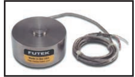
Photo 2 —The load cell uses strain gages usually in a full bridge format to measure the load applied directly to a point on the sensor.
