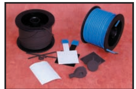
Photo 4 —QTC components from Peratech come in four basic styles: Pills, Switch Substrates, and Cable and Force Sensors. Pills can be added to current switch designs to change any push-to-make switch into a fully proportional voltage or current controller. Switch substrates can be incorporated into membrane or keypad switches to provide far greater reliability and optionally proportional control. Cable can be used in machine protection or security applications, or it can detect the presence or removal of loads. Force sensors, which offer considerably more range than standard force sensing resistors, are much more resilient to handling and environmental factors.
