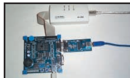
Photo 1 —I used a Keil ULINK JTAG debugger to in-circuit debug and program the LPC2138 microcontroller. I soldered an LM60 temperature sensor to the prototyping area of the MCB2130 board.
