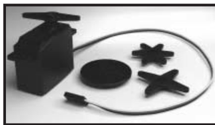
Photo 1 —A typical RC hobby servo has removable horn attachments to generate rotary or push-pull motions. Three wires are used to interface to a servo driver. Different servo manufacturers may use different wire color codes and pinouts.
