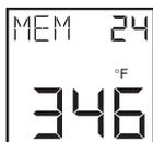
The thermometer can store up to 100 temperature data points on command. Each set of temperature data is broken down into the temperature value, emissivity, and high alarm setpoint for that temperature. This data is stored in non-volatile memory, so removing the batteries will not affect this data. To store temperature data:
