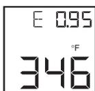
The thermometer stores the last temperature measured in the real time mode (refer to Table 2-1). This temperature can be recalled by pressing the **FUNC** key.
