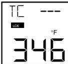
"TC--- is" is displayed when the thermocouple input is open or out of range (0 to 1600°F).
