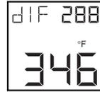
is the difference between the MAX and MIN temperatures.
