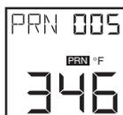
Up to 100 sets of stored temperature information can be downloaded to a serial printer or a personal computer. Each set of temperature information is broken down to the temperature value, the Emissivity, and the high alarm setpoint for that temperature.
