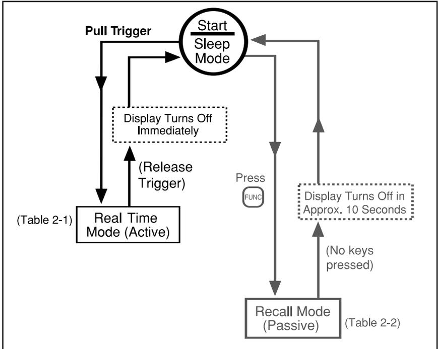
Figure 2-12. General Operational Block Diagram
