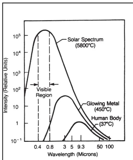
Relative emission from a blackbody versus wavelength. The area under the curve corresponds to the total energy, and is proportional to the absolute temperature to the 4th power. The peak of the spectral distribution curve shifts to shorter wavelengths as the temperature increases.
