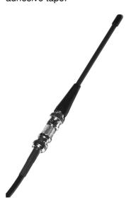
**Attention:** Always make sure to use the original cables. Other cables may have insufficient shielding or the wrong impedance (50 Ohm is required).
