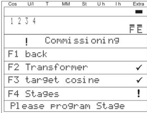
This display is used for the **Initial commissioning** of the controller, where all the necessary settings can be made.
