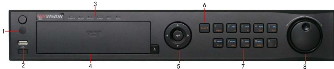
1. **IR Receiver:** operation by IR remote control.
