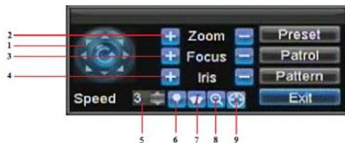
1. **Directional Pad/Auto-scan Buttons:** Controls the movements and directions of the PTZ. The center button is also used to start auto-scan of PTZ.
