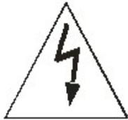
The lightning arrow symbol reminds users that there is dangerous voltage nearby, enough for a body to produce an electric shock and cause bodily harm.
