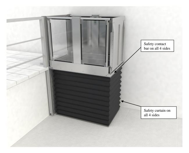
The platform is equipped with a safety curtain protection the lifting mechanism on all 4 sides. Furthermore the is a safety contact bar on the side of the upper platform floor that stops the platform in case of an obstacle being squezzed under the paltform when the platform is lowering.
