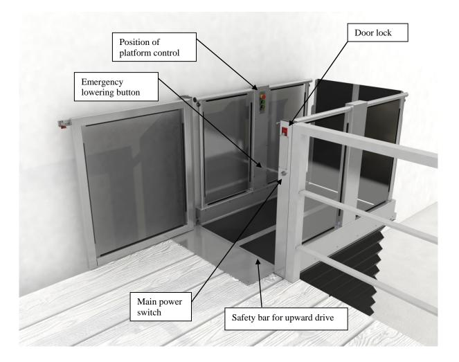
When arriving in the upper landing station the upper door lock will automatically unlock. This will allow the user to open the gate manually. Once the gate is closed again it will automatically lock again.
