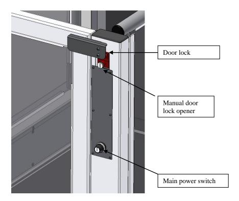
In case the door lock does not unlock electrically, it is possible to use the key to manually open the door lock and open the gate.
