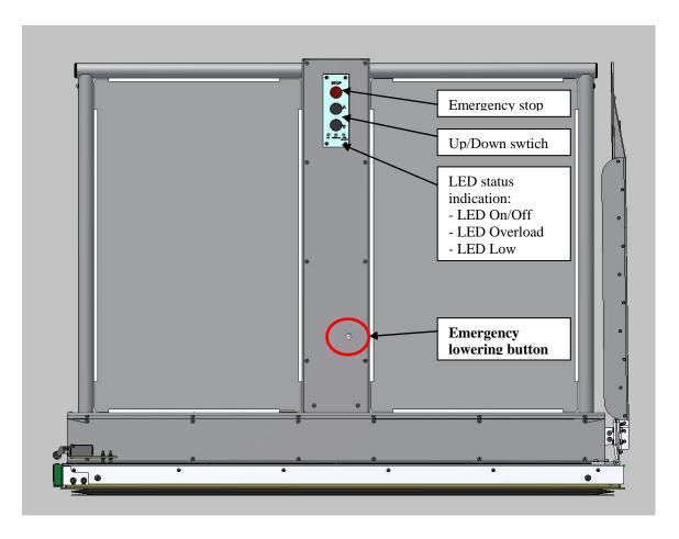
The emergency lowering button can be used to drive the platform down in case of platform malfunction. The button will also automatically open the access ramp when arriving at the lower landing area.
