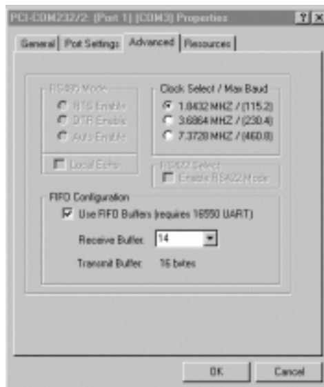
Figure 2-2. PCI-COM232 (Port1) (COM3) Properties Screen Display
