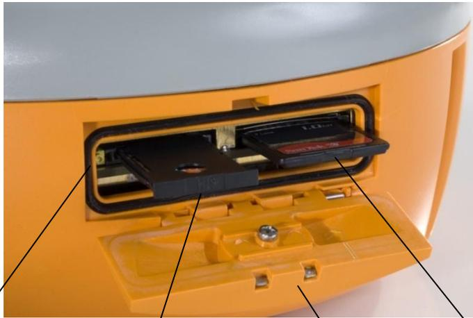
Figure 6: SIM Card & SD Card Compartment
