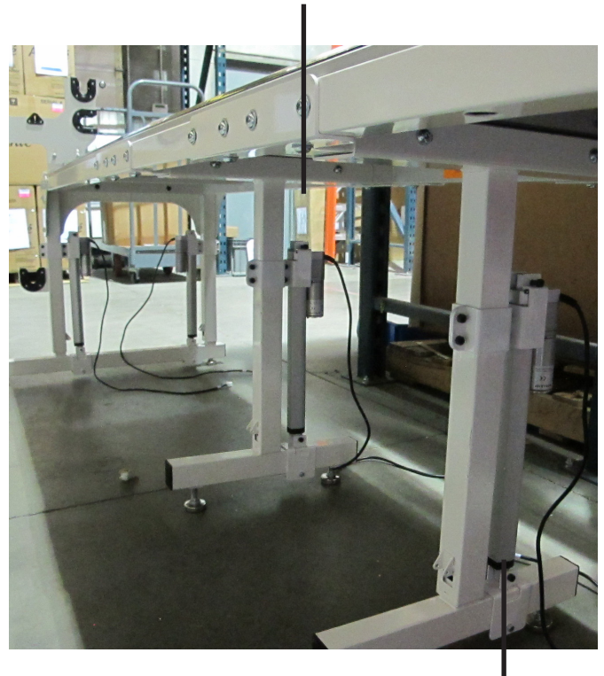
Actuator #3, mounted behind right-center leg
