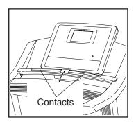
To measure your heart rate, stand on the foot rails and hold the contacts with your palms for approximately ten seconds; avoid moving your hands. When your pulse is detected, your heart rate will be shown. For the most accurate heart rate reading, continue to hold the contacts for about 15 seconds.
