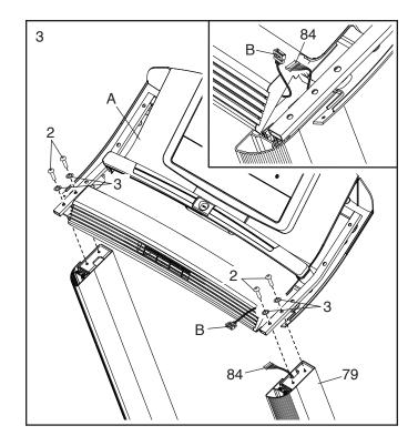
4. Connect the Upright Wire (84) to the console wire (B). See the inset drawing. The connectors should slide together easily and snap into place. If they do not, turn one connector and try again. IF YOU DO NOT CONNECT THE CONNECTORS PROPERLY, THE CONSOLE MAY BECOME DAMAGED WHEN YOU TURN ON THE POWER.
