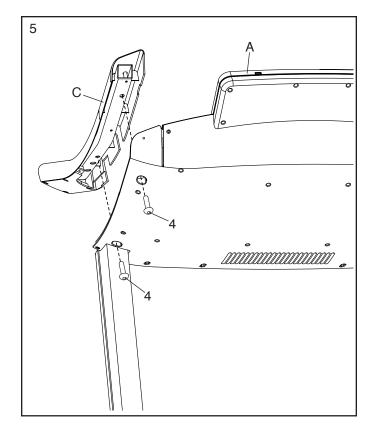
6. Tighten a #8 x 1/2" Screw (10) and a #8 x 3/4" Screw (5) into the console assembly and the right handrail assembly (C) in the locations shown. **Do not overtighten the Screws.**
