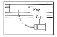
into the console. Note: It may take a minute for the console to be ready for use. IMPORTANT: In an emergency, the key can be pulled from the console, causing the walking belt to slow to a stop. Test the clip by carefully taking a few steps backward; if the key is not pulled from the console, adjust the position of the clip.
