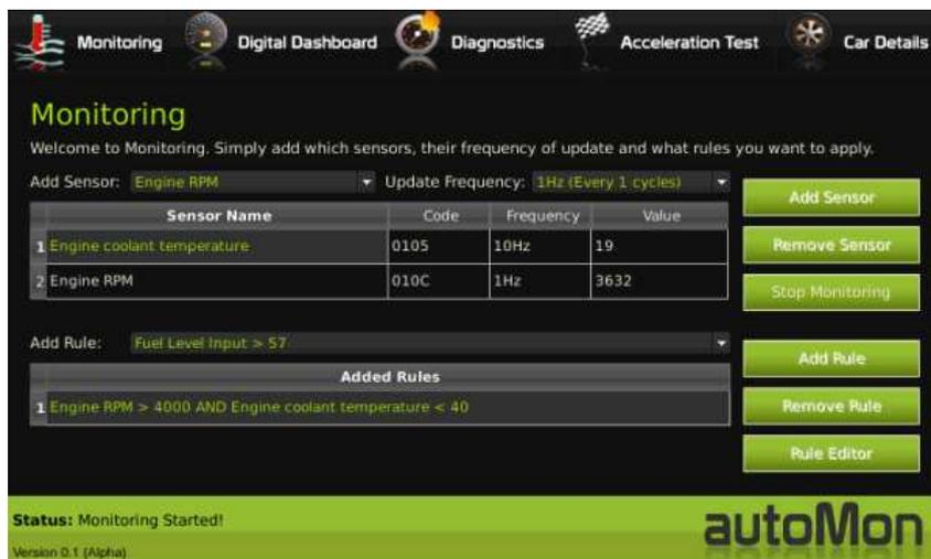
Figure 5.4 – The Monitoring section of Automon
