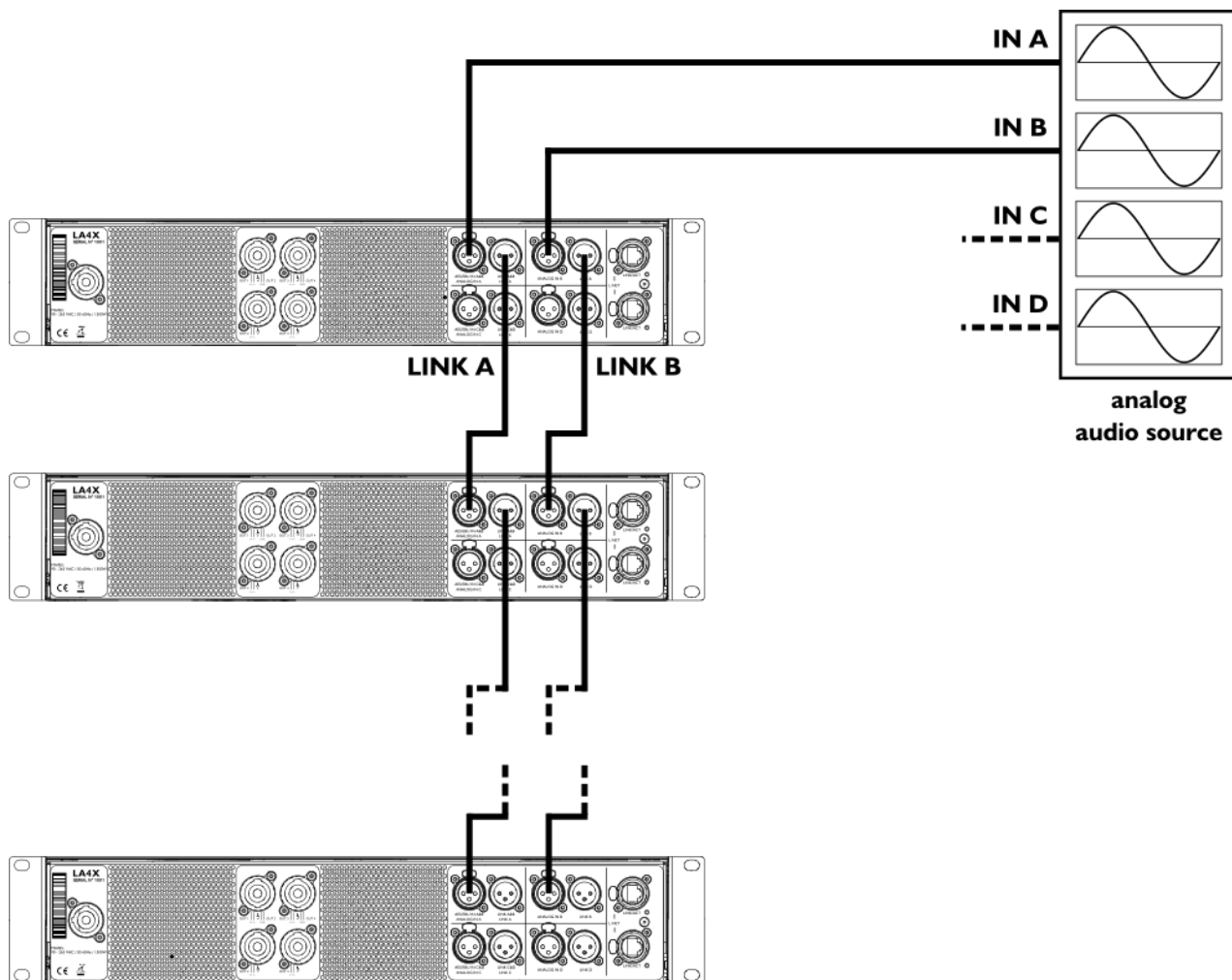
Figure 8: Daisy-chaining analog audio
