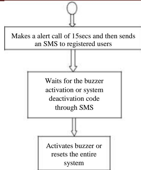
**Fig 2 : Flow diagram of Arduino task 1**
