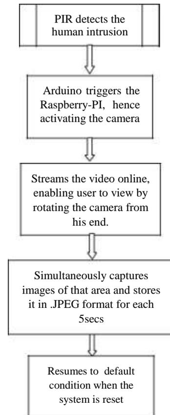
**Fig 3 : Flow diagram of Arduino task**
